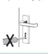
8. The deadbolt must not project when the door is in the open position.
