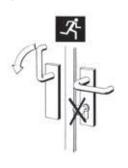
11. Panic exit devices must not be fitted with locking cylinders with knob or thumbturn.
