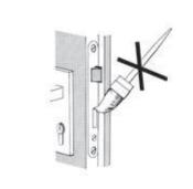
6. Do not apply any force to the lever handle other than in normal rotational direction. The maximum allowed force is 150 N.
